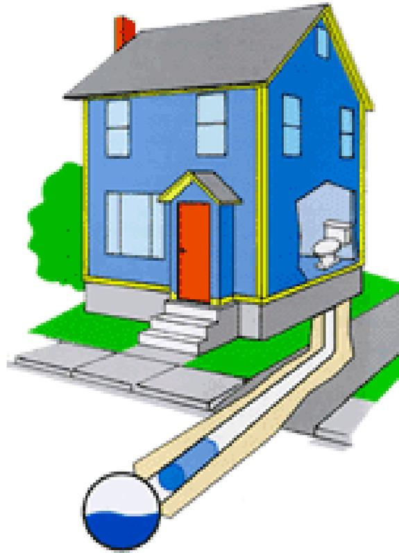
In most circumstances, these laterals were installed in an acceptable manner with state of the art materials. Over time however, the lateral pipe may crack, disintegrate, or separate at joints and allow groundwater to infiltrate into the sanitary sewer system. If the lateral is in an area with a high ground water table, the lateral may contribute a significant amount of I/I.
